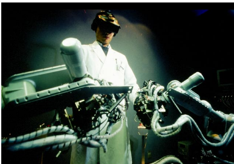
Fig. 7. A demonstration of the force feedback devices for the right and left hands.
