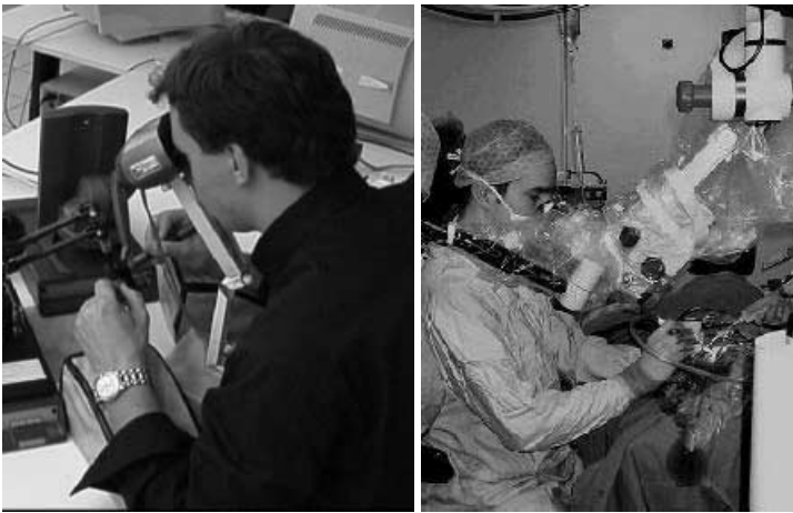
Fig. 1. Surgical simulator setup vs operating room: on the left the virtual surgical training system user interface is composed by two phantom devices that provide force feedback for sucker and burr, as well as an N-vision binocular display that presents images to the user; it simulates the real feelings of the surgeon in the operating room(right)
